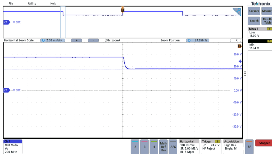
Figure 5-2: Improved Transient Performance with Dampener
